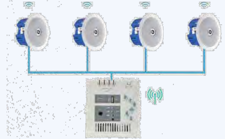
Active ceiling speaker (1 drag 4 magic box wired version) R-808
